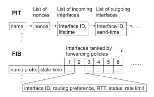
Fig. 2. Forwarding State in PIT and FIB.
