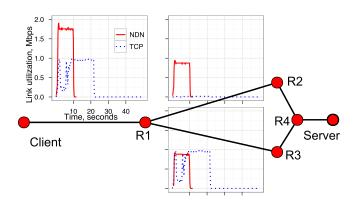
Fig. 9. Link utilization under congestion.
