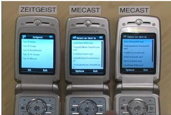
Fig. 8. Where-Fi demo showing three Motorola A-910 phones with built in WiFi support, in ad-hoc connection mode. The label above each phone describes the type of application running on the phone.
