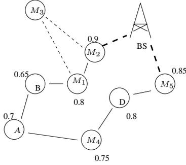
Figure 3: Example of potential attacks. A is the initiator and BS is the base station. Hosts  $M_1, \dots, M_5$  are potentially malicious. The numbers around the hosts represent their downlink rate, in Kbps. For  $\delta \geq 0.05$ , B will propagate A's request.
