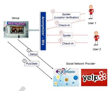
Fig. 1. Solution architecture (k = 2). The red arrows denote anonymous communication channels, whereas black arrows indicate authenticated (and secure) communication channels.
