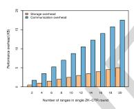
Fig. 6. Storage and communication overhead (in KB) as a function of b, the number of sub-intervals considered in the statistics computation. Even for b = 20, the storage overhead is only 5KB and the communication is 17KB.
