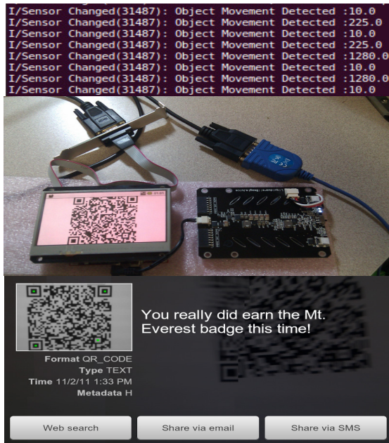
Fig. 5. FES Implementation (top-to-bottom): Detecting moving objects to enable dynamic QR-Code generation, Prototype of QR generating XACT on Beagleboard, Detecting QR-Code using off-the-shelf client software “Bar Code” scanner.
