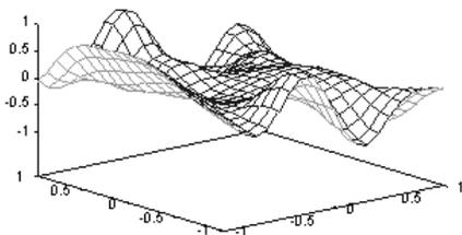
**Figure 7. The reconstructed surface after 4000 training-epochs by the robust 2-12-1 WNN**
