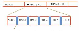
Guard time – signals transmitted by mobile terminals at different locations do not arrive at the base station at the same time
