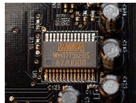
4-channel stereo multiplexed analog-to-digital converter for a sound card
