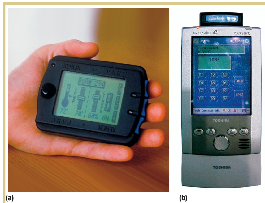
Figure 1. Hardware improvement over the last decade: (a) the Xerox ParcTab, the first context-sensitive computer (1992). The design shows the limited display available at that time—a 128- × 64-pixel, monochrome LCD. (b) a typical PDA available today with a color 240- × 320-pixel VGA (transreflective) screen.
