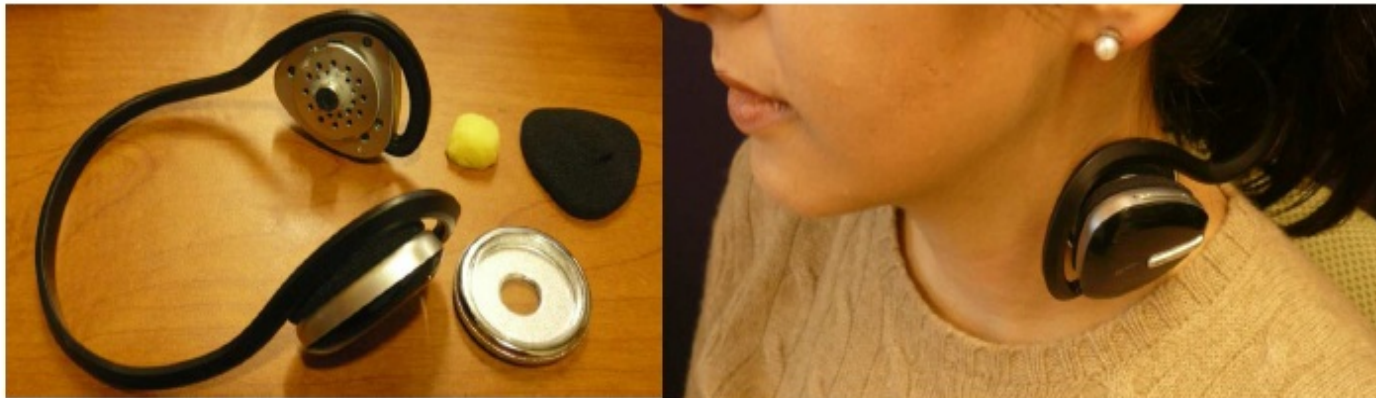
Figure 1. The BodyScope prototype. It consists of a Bluetooth headset, a microphone (embedded in the headset), and the chestpiece of a stethoscope.
