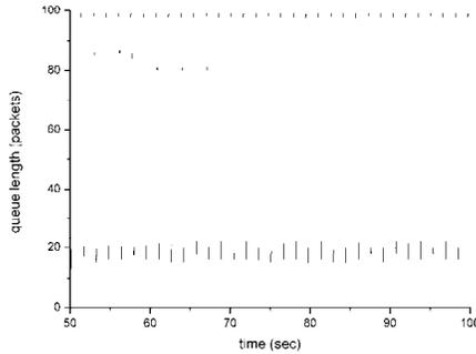
**Figure 4(c) Queue Length with TCP (1, 0.5) (DropTail gateway)**
