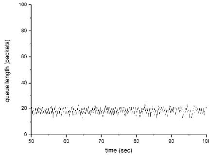
**Figure 7(a) Queue Length with TCP (0.31, 0.875) (RED gateway)**
