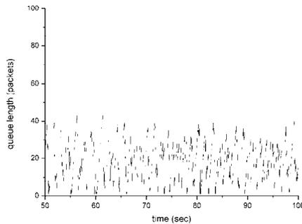
**Figure 7(c) Queue Length with TCP (1, 0.5) (RED gateway)**
