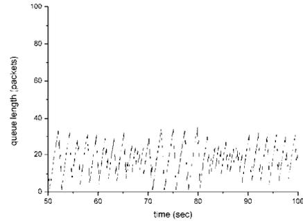
**Figure 7(b) Queue Length with TCP (0.583, 0.75) (RED gateway)**
