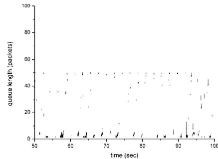
**Figure 7(d) Queue Length with TCP (1.25, 0.25) (RED gateway)**
