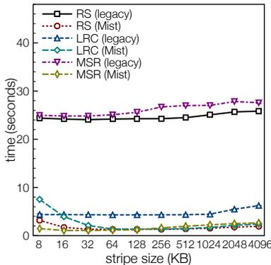
Fig. 12. The impact of the stripe size in the dissemination, with an (11, 4) Reed-Solomon (RS) code, an (11, 4, 9) minimum-storage regenerating (MSR) code and a (4, 2, 5) local reconstruction code (LRC).
