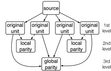
Fig. 7. The topology of a (4, 2, 1) local reconstruction code constructed in *Mist*, where there are 4 original units, 2 local parity units and 1 global parity unit to disseminate. Dashed lines represent the connections to disseminate local parity units, and other lines represent the connections to disseminate original units and the global parity unit.
