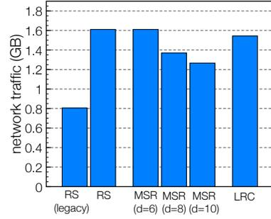
Fig. 13. The network traffic consumed in the dissemination of (12, 4) Reed-Solomon (RS) codes, (12, 4, d) minimum-storage regenerating (MSR) codes (d=6, 8, 10) and (4, 2, 6) local reconstruction codes (LRC).
