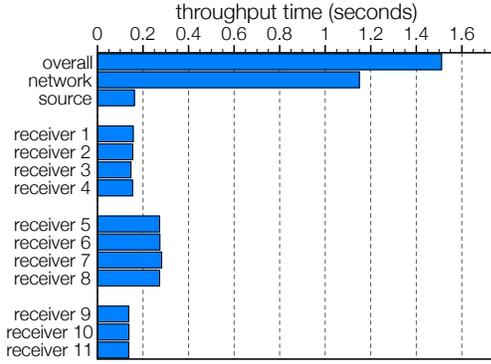
Fig. 11. A comparison of the throughput time of each component in the pipeline, with (11, 4) Reed-Solomon codes.
