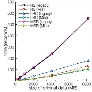
Fig. 10. A comparison of the dissemination time with original data of different sizes, with  $(8, 4)$  Reed-Solomon codes,  $(8, 4, 6)$  minimum-storage regenerating (MSR) codes and  $(4, 2, 2)$  local reconstruction codes (LRC).
