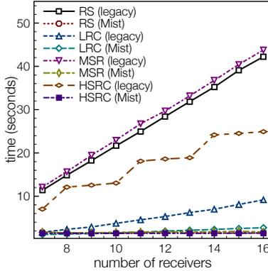
Fig. 9. A comparison of the dissemination time of  $(n, 4)$  Reed-Solomon codes,  $(n, 4, 6)$  minimum-storage regenerating (MSR) codes and  $(4, 2, n - 6)$  local reconstruction codes (LRC), with the topology in *Mist* and the legacy topology. The value of  $n$  indicates the number of receivers in the dissemination.
