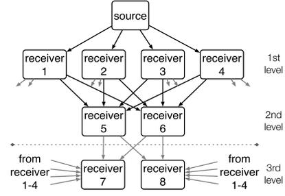
Fig. 8. An example topology for an  $(8,4,6)$  minimum-storage regenerating (MSR) codes. The source sends just 4 units of coded data to the receivers at the first level and then repair two more units in the receivers at the second level by decoding and re-encoding. From the six receivers at the first two levels, two other receivers can compute their desired data by the repair property of regenerating codes.
