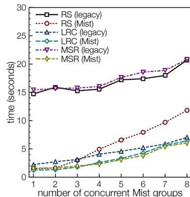
Fig. 15. The dissemination time of multiple concurrent *Mist* groups running with the same source and receivers, with  $(8, 4)$  RS codes,  $(8, 4, 6)$  MSR codes and  $(4, 2, 2)$  LRC codes.
