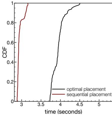
Fig. 16. The CDFs of dissemination time of the topology to disseminate data encoded with a  $(10, 8)$  RS code, with and without the algorithm proposed in Sec. 5.
