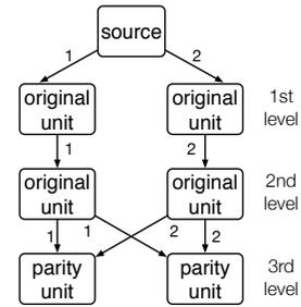
Fig. 5. The topology to disseminate a systematic  $(8,2)$  erasure code with 2-way replication of the original units. While replicating the original units at the first two levels, all other (*i.e.*, parity) units are disseminated in the same way as the topology for general erasure codes.
