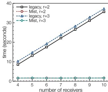
Fig. 14. The dissemination time of a systematic  $(n, 3)$  RS coded data with an  $r$ -way replication of original units, where the value of  $n$  indicates the number of receivers of coded data in the dissemination, excluding the additional receivers of replications.
