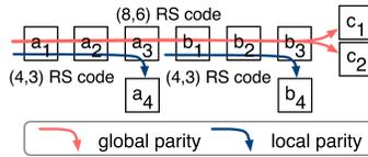
Fig. 6. An example of (6,2,2) local reconstruction codes, with 6 original units, 2 local parity units and 2 global parity units.
