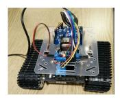
motors. A L298N dual channel H-bridge is used for the control of the motors. It receives some 3.3V signals of the Wemos board, and provide higher voltages for the
