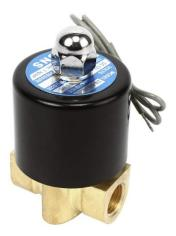
Water valve that is controlled through electric currents. The valve is closed normally, but when a current is provided the valve opens and allows water to flow through.
