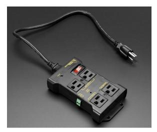
This relay outlet allows for relay control of an outlet and thus for control of any light source connected to that outlet. This mechanism is for the purpose of providing additional light to the plant as seen necessary.
