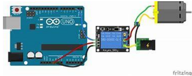
Figure 4: Connection of Arduino and relay to water pump
