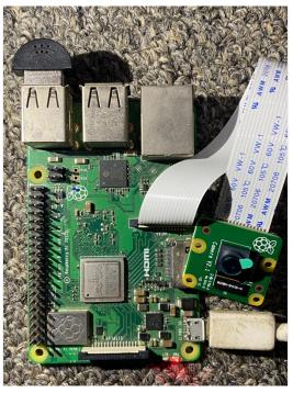
2.1.1 Raspberry Pi. We have used Raspberry Module as our computation device which hosts our software and collects reading from attached peripherals and performs actions based on set condition. Processor speed ranges from 700 MHz to 1.4 GHz for the Pi 3 Model B+ or 1.5 GHz for the Pi 4; on-board memory ranges from 256 MiB to 1 GiB random-access memory (RAM), with up to 4 GiB available on the Pi 4..
