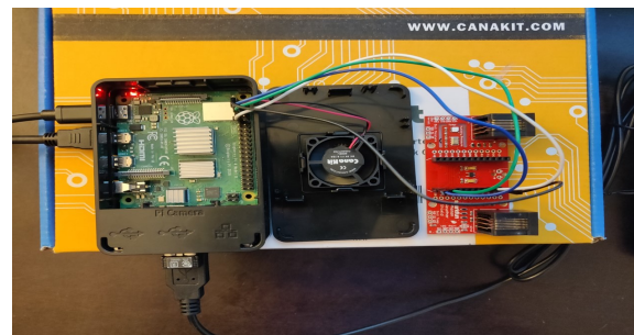
Figure 2: Raspberry Pi 4 connected with Sparkfun Photon Weather Shield
