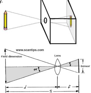
We used trigonometry to calculate the distance between the camera and user. Since we knew all parameters we need, we can get the distance by this formula.
