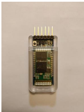
Figure 3:Bluetooth HC-05 module
