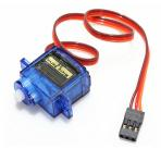
The nodemcu acts as my main logic board and it's responsible for sending and receiving data from the web server to the application as well as controlling the servo motor behaviour. The HCSR04 ultrasonic sensor is used to calculate the remaining water amount inside the water tank of the coffee maker. The servo motor is used to trigger the coffee maker controls and start the device.
