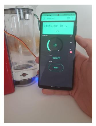
As can be seen in the image above the HCSR04 correctly measures the water distance and then sends the data to Nodemcu. The data then is processed in the Nodemcu and used to calculate the remaining water percentage which is then sent to the application display via the web server.
