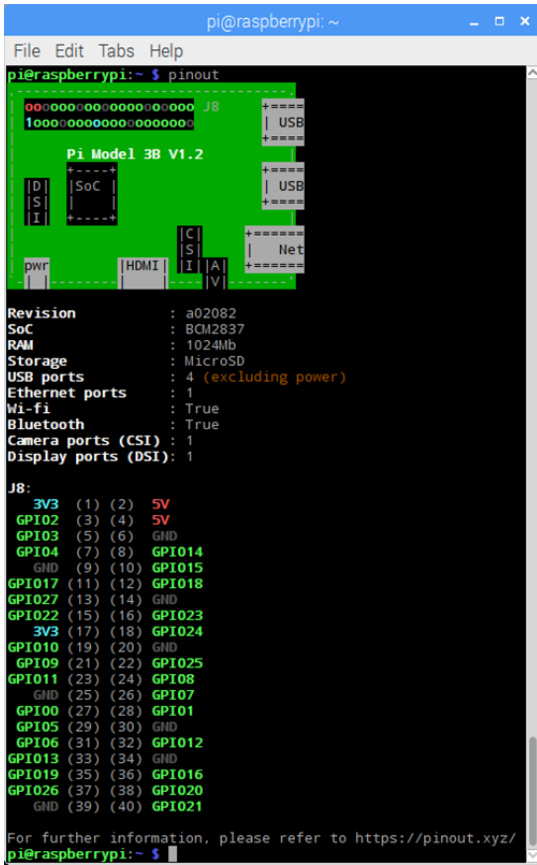
Fig. 3. GPIO Pins for Raspberry Pi
