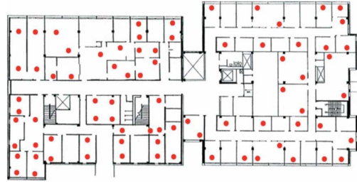
Fig. 3. Testbed in Bryan and Jolley Hall of Washington University in St. Louis. Red dots indicate the sensors.
