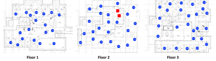
Fig. 12. The deployment of CPSL Testbed. Blue circles denote sensors and actuators and red squares represent two access points.
