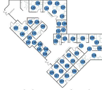
Figure 4: Testbed consisting of 50 TelosB motes.
