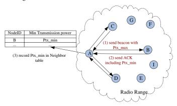
Figure.2. Operation of transmission power control
