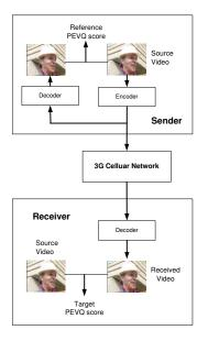
Fig. 2. The procedure of measuring PEVQ score ratio.
