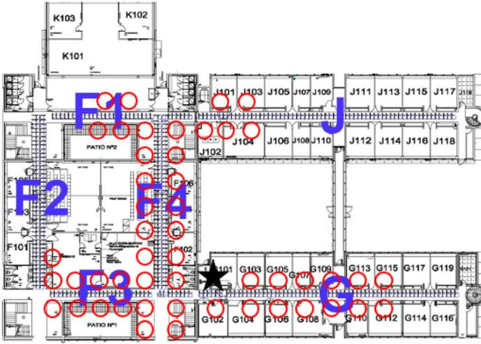
Fig. 2. Testbed used for our studies. All 50 devices are deployed on the same floor in an office building. The black star indicates the device that serves as the border router (Root) and the read circles denote end devices.
