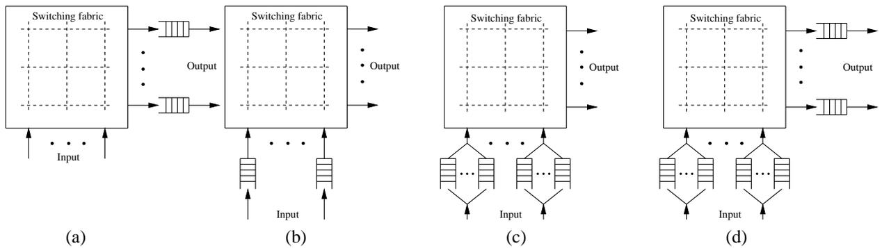
Fig. 1. Packet switches can be divided into different categories by the location where the blocked packets are buffered. (a) Output queued switch. (b) Single input queued switch. (c) Virtual output queued switch. (d) Combined input output queued switch.
