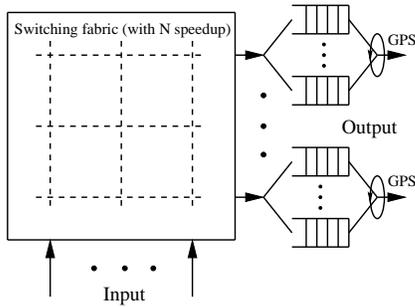
Fig. 3. The ideal model for per port multicast fair scheduling is based on the output queued switch, and each output port runs the GPS scheduler to ensure the fair bandwidth allocation.
