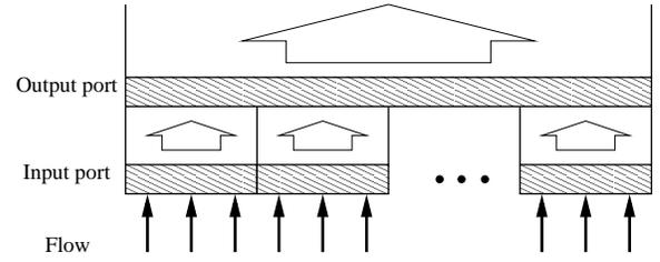
Fig. 2. The per flow fair scheduling for packet switches can be decomposed to two levels: the per port based fair scheduling and the per flow based fair scheduling.
