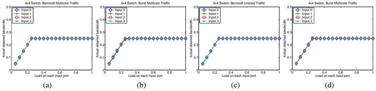
Fig. 5. FIFOMS is not able to provide bandwidth guarantee. (a) Actually obtained bandwidth under Bernoulli multicast traffic. (b) Actually obtained bandwidth under burst multicast traffic. (c) Actually obtained bandwidth under Bernoulli unicast traffic. (d) Actually obtained bandwidth under burst unicast traffic.
