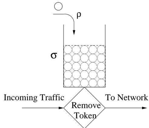
Fig. 2. A leaky bucket has a token bucket of capacity  $\sigma$  with new tokens flowing in at rate  $\rho$ .
