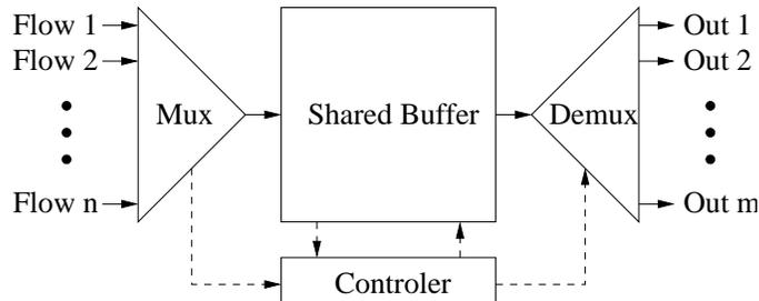
Fig. 1. The shared buffer switch may have a single or multiple outputs. Among the incoming flows, some are guaranteed performance flows that require lossless service.
