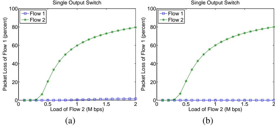
Fig. 5. The buffer allocation for lossless service in the packet switched network needs to be adjusted due to packet fragmentation. (a) Packet loss before adjustment. (b) Packet loss after adjustment.
