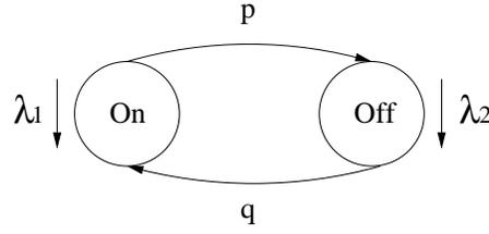
Fig. 4. In a Markov modulated Poisson process, the intensity of the Poisson process depends on the state of the Markov chain.
