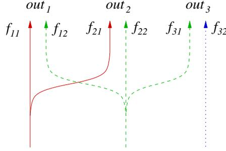
Fig. 3. A physical multicast flow may be labeled as different flows at different outputs.
