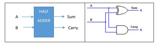
Show how to connect two Half-Adders to form a Full-Adder (You will need an OR-gate) Hint:  $A + B + C_{in} = (A + B) + C_{in}$
