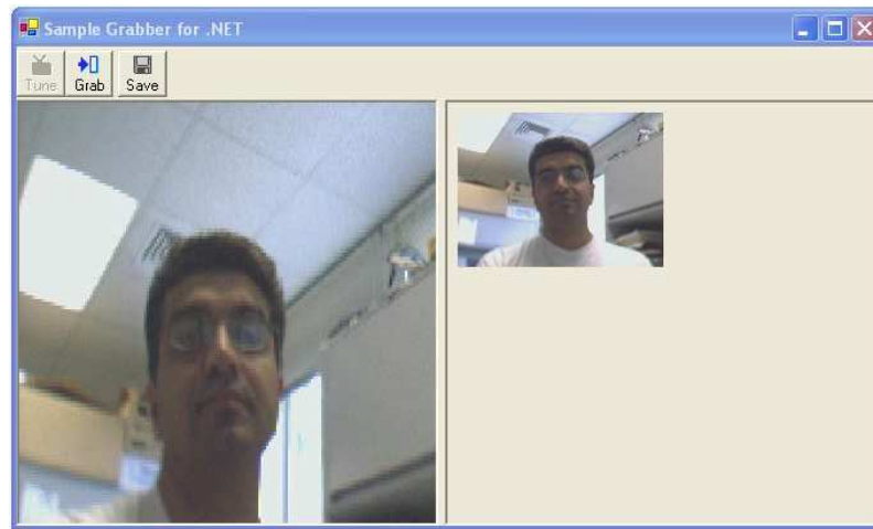
Figure 6.10: A screen dump of the sample grabber application GUI. The left panel shows a preview of the live video captured from a video camera and the right panel shows a still image grabbed using the “Grab” toolbar button.
