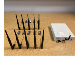
Fig. 5. LoRa Transmitters and a USRP Receiver.
