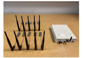
Fig. 5. LoRa transmitters and a USRP receiver.
